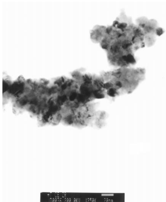
Fig. 8 Transmission electron micrograph (TEM) of \text{Ce}_{0.47}\text{Zr}_{0.53}\text{O}_2 after calcining at 1000 °C for 1 hour (bar = 20 nm).
